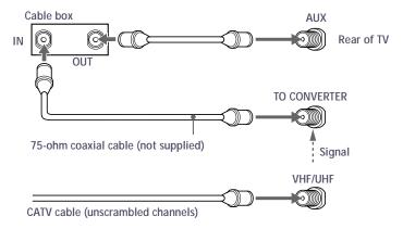
To switch between channels from Cable Box and channels coming directly into TV
